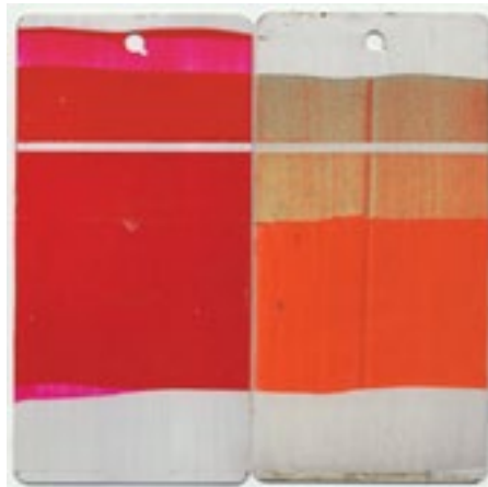
Fluorescent Magenta. 10 mil. Uncoated, with Isolation Coat, and with 2 coats MSA Varnish. Left is unexposed, right after 1 year exposure.
