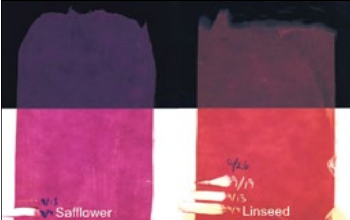
Image 1 – 3 mil drawdowns of Cobalt Violet Light in Linseed and Safflower after 2.5 years of dark aging.
