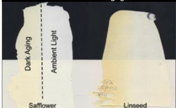
Image 3 – 3 mil. Drawdowns of Flake White with half of each card being covered after drying.
