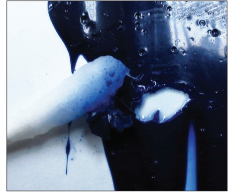
Heavy Body Phthalo Blue (Red Shade) mixed 1:1 with Retarder 50 mil drawdown showing water sensitivity after 1 week cure at 75°F, 40% Relative Humidity
