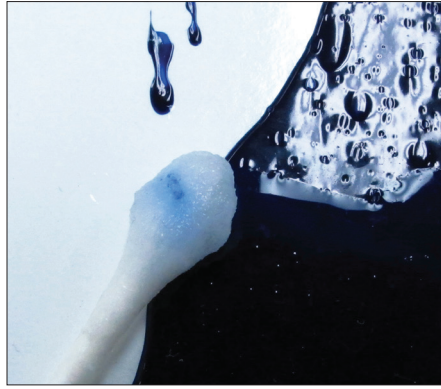
Heavy Body Phthalo Blue (Red Shade) mixed 8:1 with Retarder 50 mil drawdown showing water sensitivity after 1 week cure at 75°F, 40% Relative Humidity
