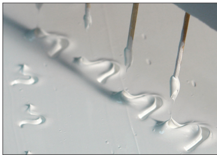
Figure 4 - Toothpick comb used to manipulate hours-old gel cast at 1/4" on acrylic sheeting.
