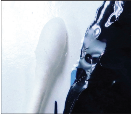
Heavy Body Phthalo Blue (Red Shade) 50 mil drawdown showing water sensitivity after 1 week cure at 75°F, 40% Relative Humidity
