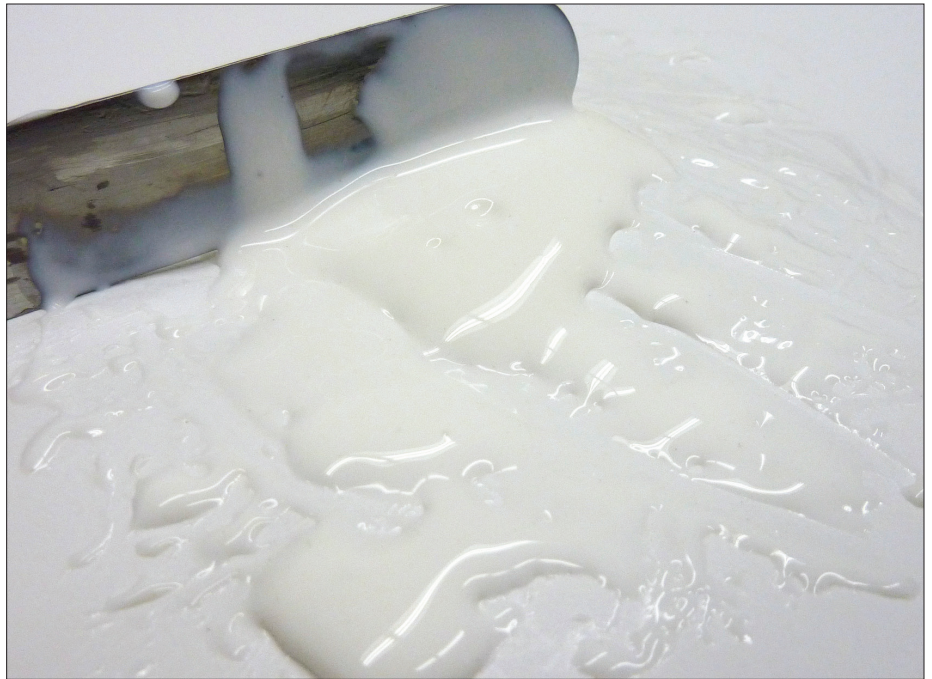
Thick Self Leveling Gel agitated with a palette knife, relaxes after several minutes, losing all tool marks.
