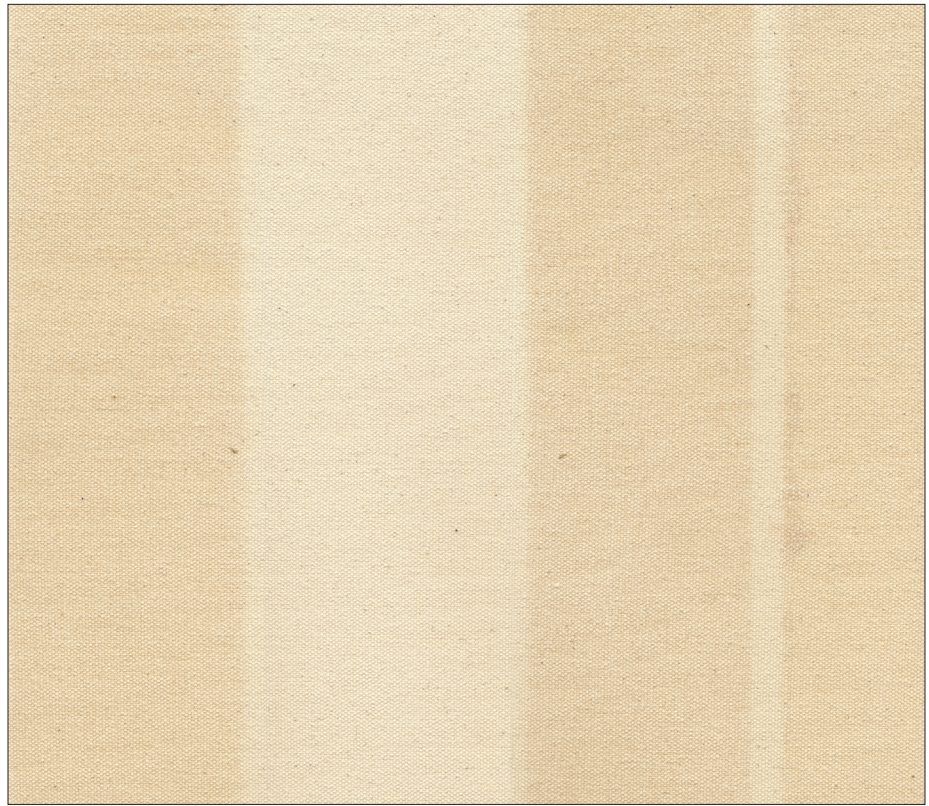
Testing for strikethrough of oil ground on top of a size. Dark areas on back of canvas show where oil from the ground has penetrated through.
