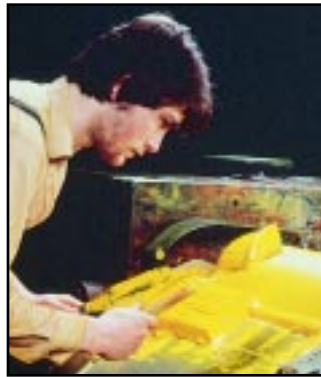
Oil colour milled on a traditional, triple-roll mill at the Winsor & Newton factory.
